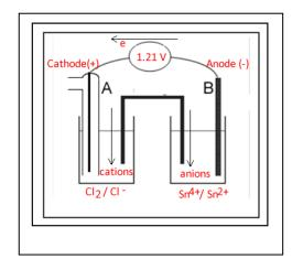
b) What are electrodes A and B made from? *Graphite or Pt* What properties should these material have in order to be used as electrodes in this galvanic cell? *Must conduct electricity and be inert*
